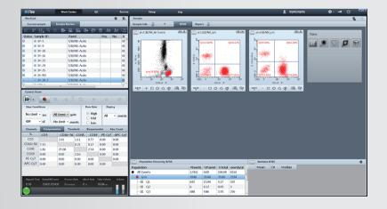
BriCyte E6 can gate the populations of cells by the built-in algorithms, then it analyzes the data and reports the results automatically. Currently this feature is for Mindray reagents only.
