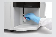
BriCyte E6 has open mode which suits the labs which have less number of samples, the micro sample tubes are supported as well. The carrousel mode is yet another option which can handle 40 sample tubes at one time.
