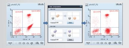
BriCyte E6 can perform automatic compensation by one simple click of the built-in intelligent template.
