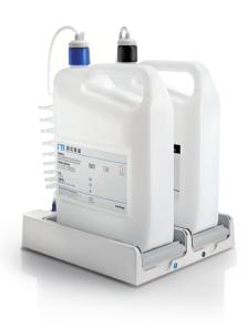
The sheath fluid and waste could be placed on the weight sensors which are able to measure the residual volume of reagents. With such design, the BriCyte E6 can sound an alarm before the reagents run out to minimize the dead volume.
