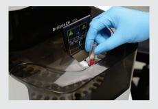
In the carousel mode, single sample tube can also be loaded as STAT after opening the cap of carrousel.
