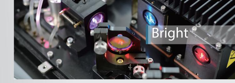
BriCyte E6 is equipped with dual-laser based optics. A red diode laser and a blue diode laser are used for exciting 4 to 6 colors of fluorescence lights. The optics are designed with state-of-the-art technology to ensure higher sensitivity for a better identification of cellular populations.
