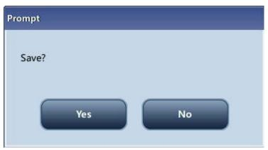
Tap "**Yes**" to save the settings and switch to the corresponding screen. Tap "**No**" to switch to the corresponding screen without saving the settings.
