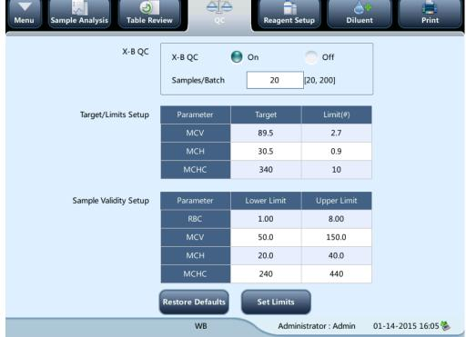
On the X-B QC setup screen, you may activate/deactivate X-B QC, set target/limits, and configure the sample validity setup.
