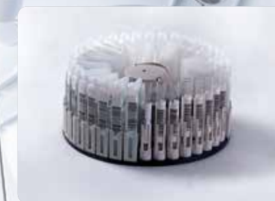
Refrigerated sample/reagent disk
