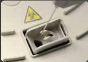
Waterfall probe cleaning
