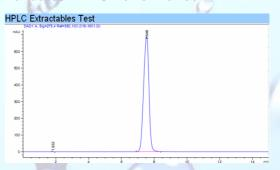
Agilent Technologies 1200, Column: C18 UV = 254 nm Mob.phase:MeOH/H<sub>2</sub>O:20:80, Temperature: 25 °C, Flow rate:0.8ml/min, sample:2mg/ml Bergenin(in Methanol)
