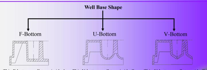
This F-bottom well type is ideal for precise optical measurements.
